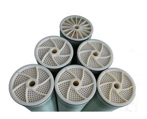
HYDRONANO Industrial LPRO membrane element is developed for energy saving applications with low operation pressure. It has the characteristics of high flow and excellent rejection performance in salt rejection. It is especially suitable for the preparation of ultra pure water in Pharmaceutical, Electronics and Power industry etc. DeltaPure LPRO8040 has large filtration area of 37m2 with 99.5% stable salt rejection rate.
